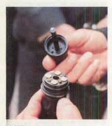
ABOVE: Load pistol with four .22LR cartridges. Three of four firing-pin holes can be seen here inside pommel unit.
